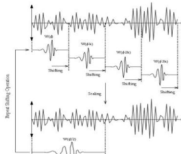
Fig. 2 Scaling and Shifting process of Discrete Wavelet Transform
