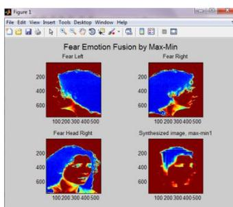
Fig. 6 Fear emotion fused by Wavelet Transform MaxMin decomposition
